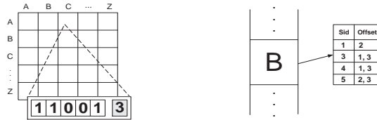
Figure 1. (a) Content of the pair A \rightarrow C in the Bitmap Matrix; (b) Representation of event B in the Offset Matrix
