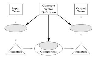
Figure 2.2: Architecture for *concrete syntax* meta-tools. The concrete syntax definition serves as contract between components. Components that import generated library code interoperate with each other and with generated parsers and pretty-printers by exchanging parse trees adhering to the contractual grammar.
