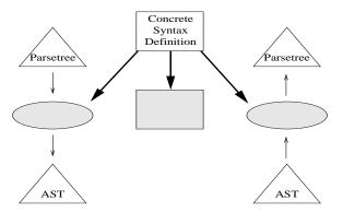
Figure 2.6: Architecture for meta-tools linking abstract to concrete syntax. The abstract syntax definition is now generated from the concrete syntax definition.
