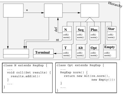
Figure 1.8: UML diagram of the class hierarchy for the EBNF syntax. The Java implementation of the methods coll() and norm() are shown only for the 'interesting' cases.
