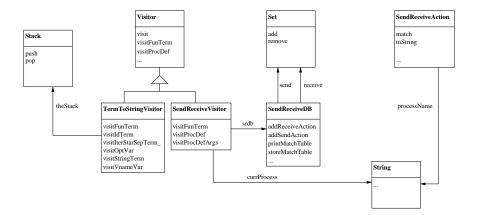
Figure 6.12: UML diagram of the ToolBus analyzer.
