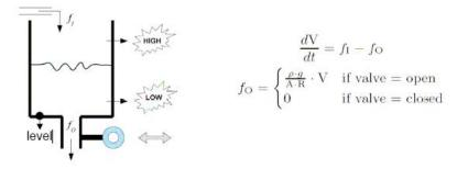
Figure: The water tank example
