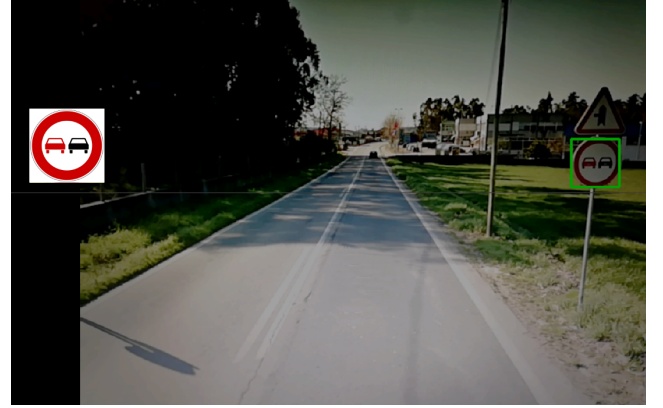
Fig. 10: Example of the detection phase missing a sign when multiple signs are present
