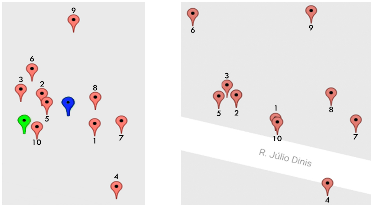
Figure 28.: Left: Sign computed locations (pink), mean value (blue) and sign real location (green); Right: Vehicle GPS location
