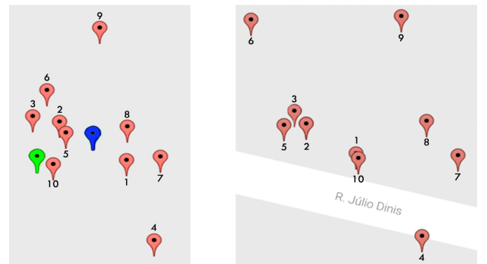
Fig. 11: Left: Sign computed locations (pink), mean value (blue) and sign real location (green); Right: Vehicle GPS location
