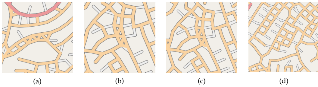
Figure 79: Images obtained from a single road map: a-c) Triangular connections; d) Perpendicular connections.
