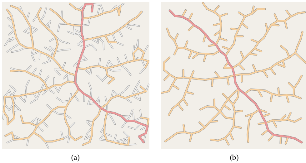
Figure 83: a) No validation; b) Validation used, safety distance as half of segment length.
