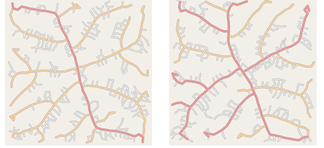
Figure 7: Automatic road hierarchy: red primary ; yellow secondary; grey:tertiary roads.
