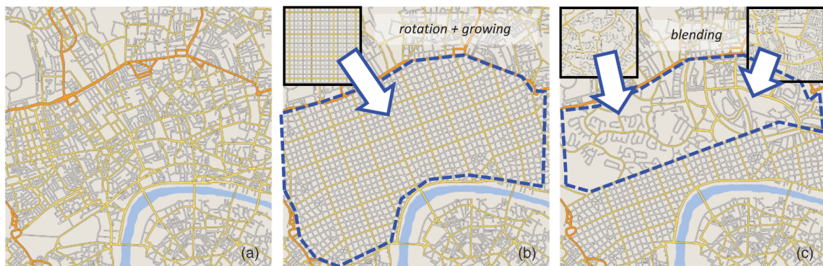
Figure 61: a) User-selected target area; b) Area replaced with a regular grid pattern; c) A more organic type of network was generated in the centre. Source: Nishida et al. (2016)
