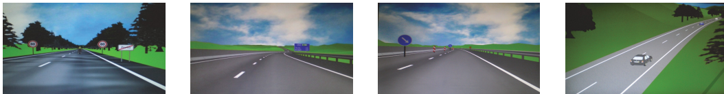
Figure 58: 3D Results showing the generation of both vertical and horizontal signalisation in both urban and rural environments. Source: Campos (2015)
