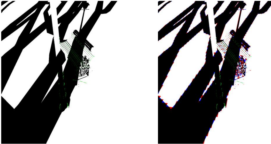
Figure 79 - With-Bench scene with a 1024x1024 viewport and 1024x1024 shadow map; (Left) OptiX Prime results; (Right) NSM results; Blue pixels represent the incorrect light pixels, and red pixels represent the incorrect shadow pixels.
