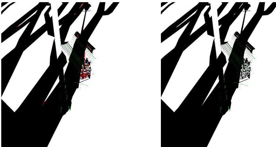
Figure 93 - With-Bench scene with a 1024x1024 viewport and 1024x1024 shadow map; (Left) PCF results; (Right) CRSM/CRSMA results; Blue pixels represent the incorrect light pixels, and red pixels represent the incorrect shadow pixels.
