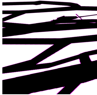
Figure 46 – PCF's "uncertain" pixel detection. The purple pixels represent the "uncertain" detected. Viewport size 1024x1024 and Shadow Map size 2048x2048.
